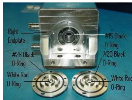
Figure 5-2 No Retainer Cap Version O-rings
